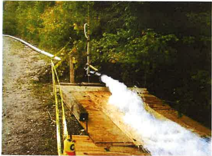
Discharge during a pumping test of one of two, 2,000 gpm production wells HSA sited and developed for the Village of Malone, NY
