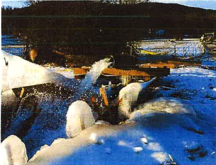
Discharge of 1,500 gpm During Pumping Test of a New Well HSA Sited and Developed for Ticonderoga, New York
