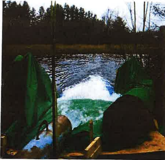
3,000 gpm discharge during pumping test of a new well HSA sited and developed for Saranac Lake
